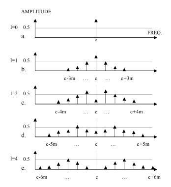
Fig. 1. Example to show increasing bandwidth with increasing modulation index, 1. The upper and lower side frequencies are at intervals of the modulating frequency, m, and are symmetrical around the carrier, c.
