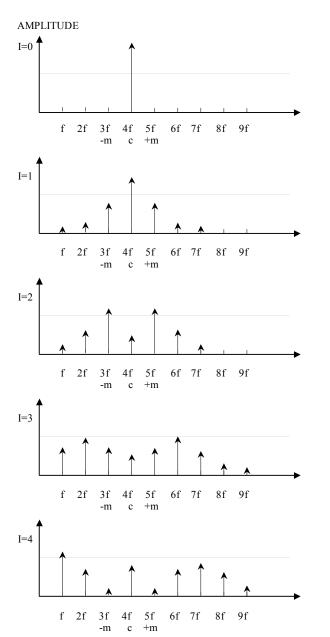
Fig. 5. Plot of spectrum where the ratio of c/m is 4/1. As the index increases, the reflected lower side frequencies begin to affect the spectrum when I = 3, where the fundamental, c—3m, is noticeably greater than the 7th harmonic, c+3m.
