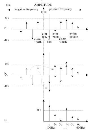
Fig. 4a. shows the spectrum with components that lie in the negative frequency domain; b. shows a plot from a. in which the frequencies in the negative domain are reflected around 0 Hz with an inversion of phase and added to the components in the positive domain; c is plot of the magnitude of the components of b.
