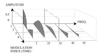
Fig. 7. Dynamic spectrum where the ratio c/m = 1/1 and the modulation index increases from 0 t o 4 continuously. The increasing bandwidth of the spectrum is clearly seen, but because of the reflected side band frequencies, the evolution of the individual components is not intuitively clear.
