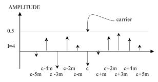
Fig. 3. Plot of Fig. le with phase information included (modulation index = 4). The bars extending downward represent spectral components whose phases differ by  $180^{\circ}$ .
